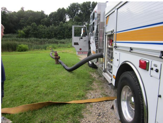
All set up and ready to draft. The hydrant in the foreground is an out of service hydrant.
