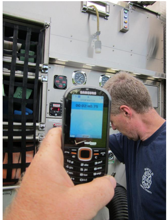
Test #1 = 2:40 minutes - prime to pump pressure time!
