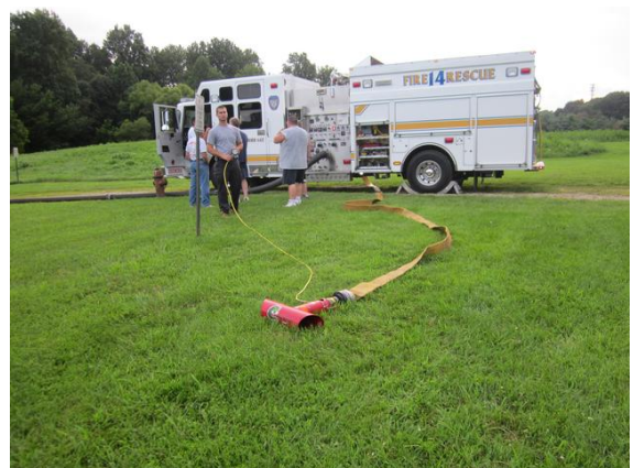
The flow measurement set-up.
