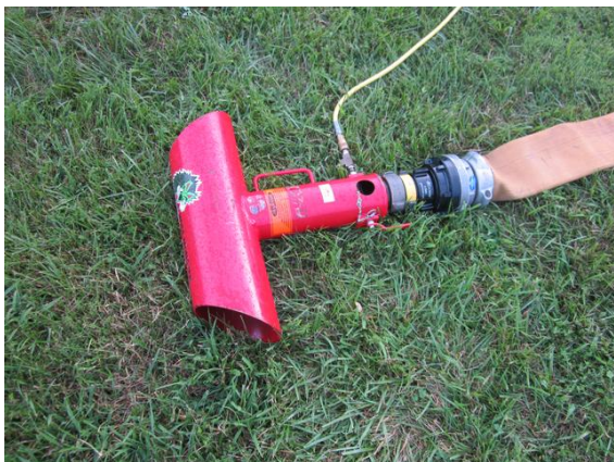
A HoseMonster flow diffuser with built-in pitot was used to measure the flow.
