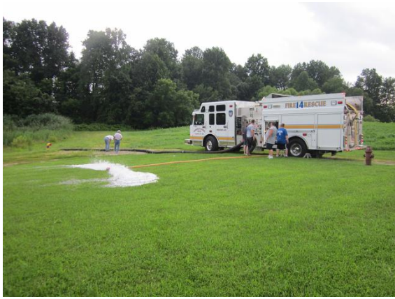
Winfield VFD E142 drafts through 100-feet of 6-inch suction hose using its new, automatic air primer.
